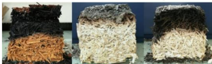
Different kinds of biobased concretes after cone calorimeter tests
